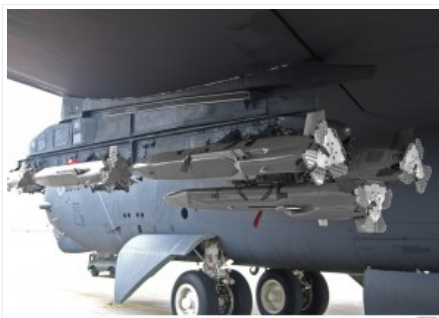
MALDs on the port inner pylon of a B-52. Unlike the MALD-J jammer variant of the MALD, NGJ is intended to take on a wide range of jamming tasks. Photo courtesy of Raytheon
